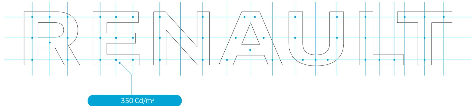
The dots are a schematic representation of the measurement points that should present similar light intensity values in order to obtain even lighting across each of the letters of the Renault word.
